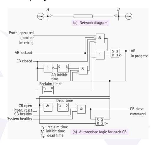
In the example above, if it were decided to charge the line initially from station A, the dead time in the auto-reclose relay at A would be set at, say, 5 seconds, while the corresponding timer in the auto-reclose relay at B would be set at, say, 15 seconds. The circuit breaker at A would then reclose after 5 seconds provided that voltage monitoring relays at A indicated that the busbars were alive and the line dead.
